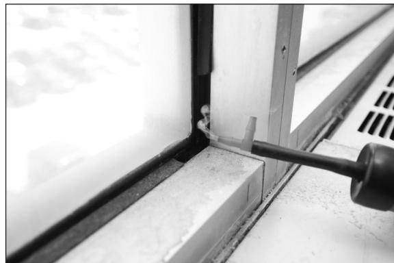
smoke pencil. Sometimes a large-scale depressurization fan is used to create negative pressure in the building and increase the visibility of leaks. In some instances, infrared thermography from outside the building can show patterns of air leakage. Energy saving potential is analyzed using EC 128/ALCAP software.
